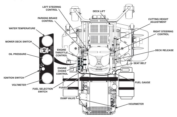
Figure 4-1. Controls and Instruments
